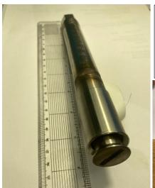
The anchor is 20cm long and just 2.5cm diameter. The top section of the anchor can be unscrewed to become proud of the road surface. A flat black plate then slots over and the tightened back up. The gazebo can now be strapped down to the anchor.
